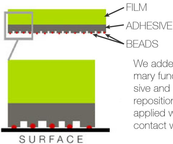
We added small beads on the surface of the adhesive. Their primary function is to limit the surface interaction between the adhesive and the target surface. This innovation allows for enhanced repositioning, sliding and placement of the film. Once the vinyl is applied with pressure, the beads break, allowing the adhesive full contact with the target surface.
